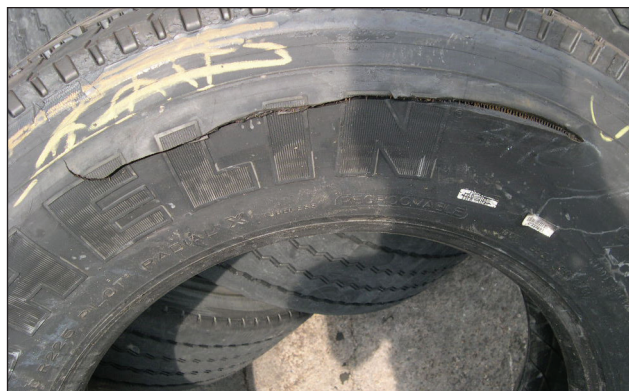
Fatigue Rupture or “Zipper”
